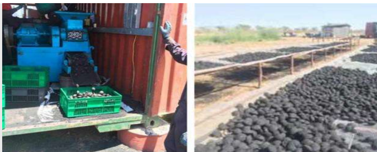
Figure 3: Briquette production in Kakuma Refugee Camp, Turkana, Kenya. Left: Mechanical press producing briquettes from treated sludge and waste biomass. Right: Drying of briquettes (source: Sanivation)
